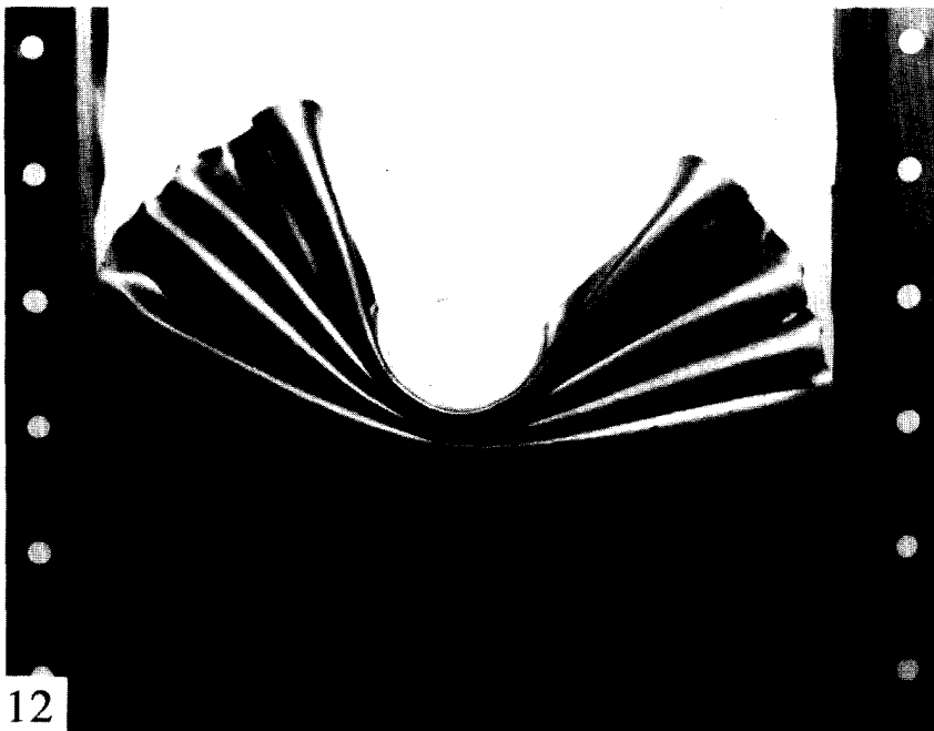
Fig. 6. A concertina tearing mode with two diverging cracks originating from a local cut.
